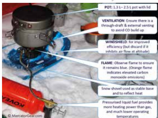
FIGURE 1 ABOVE Stove selection is driven by the Temperature-Altitude Profile for a given type of expedition. RIGHT Snow melting setup for three people at altitude: liquid fuel configuration. © MercatorGear.com. FAR RIGHT Jetboil.
