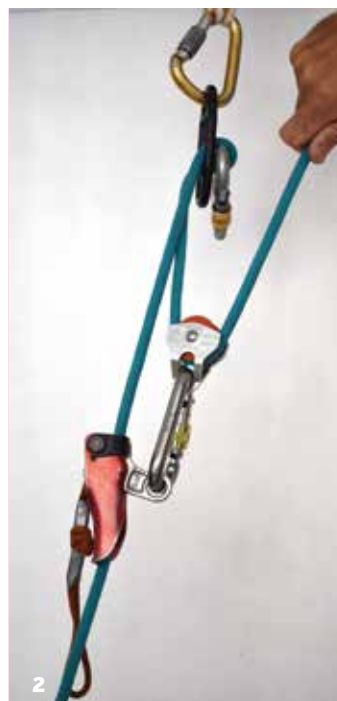
1. Kong GI-GI in use (left) and Original New Alp in use (right). © Simon Powell. 2. My hoist kit: Shunt and pulley haul – lighter gadgets are now available! © Simon Powell.
